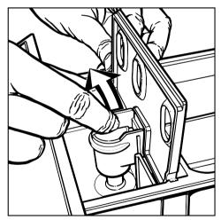
Remove the suction tube from compartment <sup>(a)</sup>, wash under running warm water and replace.
